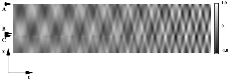
FIG. 3. The transition behavior of the system in Eq. (1) is plotted in a space-time diagram (horizontal time, vertical space). The originally stable spatiotemporal pattern is destabilized by moving the location of the heterogeneous projection from x_2=B to x_2=C . The units used are the number of time steps and the arbitrary amplitude, respectively.
