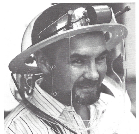
Scott Kelso wearing helmet designed to provide visual feedback of speaker's vocal track events.
